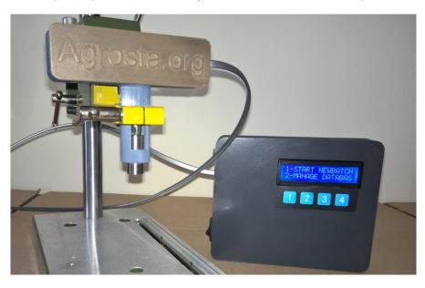
The devices takes the origin when you switch it on. If the sensor is not in the right position when you start the device, you can have a mistake in the measurements that can reach up to the weight of the tip + stainless shaft (50 grams)
