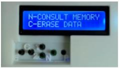
Press 3 for batches consultation – Each batch statistics is displayed during 3.5 seconds – "A" corresponds to the average, "St" is the standard deviation of the batch, "Hi" corresponds to the homogeneity index of the batch (shall be less than 10% for good homogeneity)
