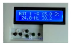
Press 1 to erase Data, and go back to Batch 1, the data is deleted on SD card (Confirmation is asked by pressing 2)
